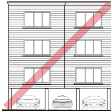
Figure 5-65. Building appears to float over the parking.
