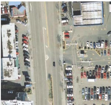
Figure 5-49. Inadequate throat depths for every driveway.
