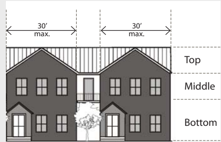
Figure 6-10. An example sketch of a multi-story building that meets the articulation standards.
