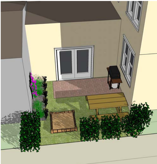
Figure 7-46. For zero lot-line homes, a 15x15 space is the minimum size necessary to fit desirable yard elements, such as a picnic table, barbeque, sandbox/play area, and some landscaping.
