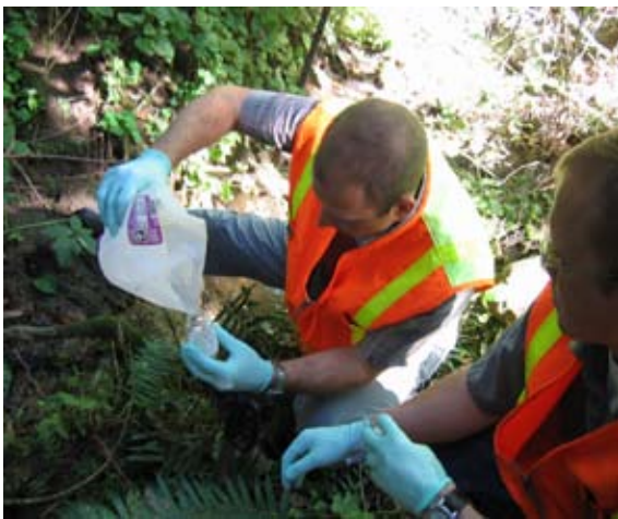
Top: Checking for potential illicit discharges. Bottom: Staff sample a suspected illicit discharge.
